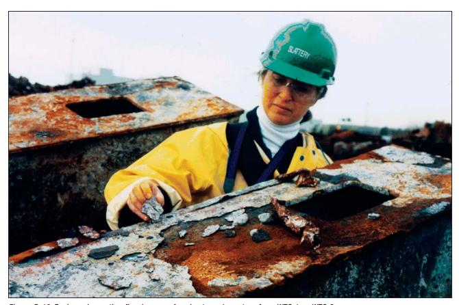
Figure D-16 Engineer inspecting fire damage of perimeter column tree from WTC 1 or WTC 2.
