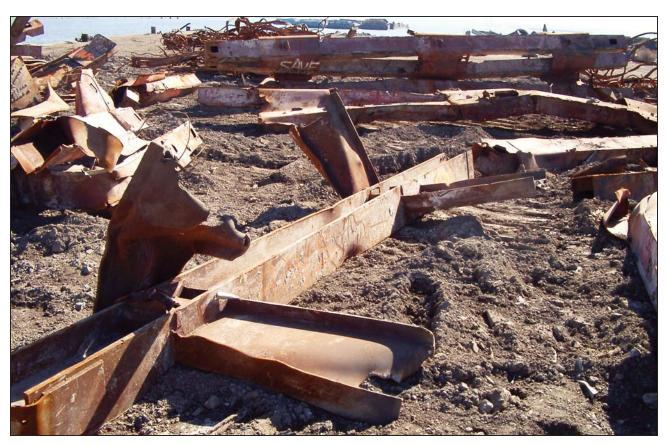
Figure D-14 WTC 7 W14 column tree with beams attached to two floors.
