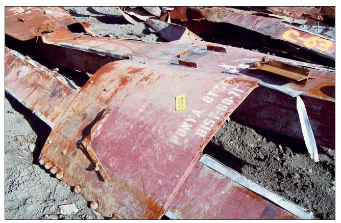
Figure D-5 Stenciled markings on WTC 2 perimeter column from floors 68-71.
