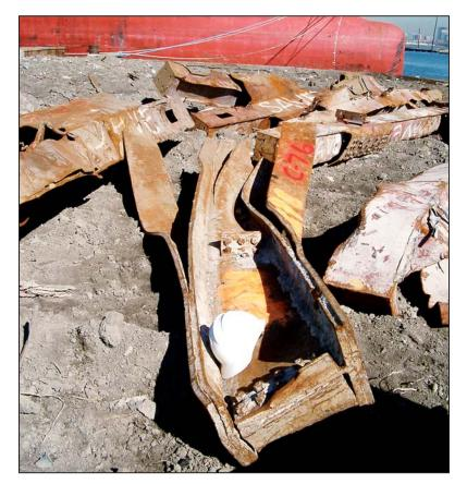
Figure D-15 Built-up member with failure along stitch welding.
