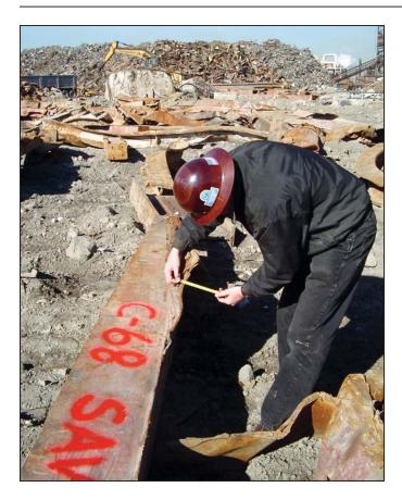
Figure D-8 Engineer measuring spandrel plate thickness  $(t_{\rm s})$ .
