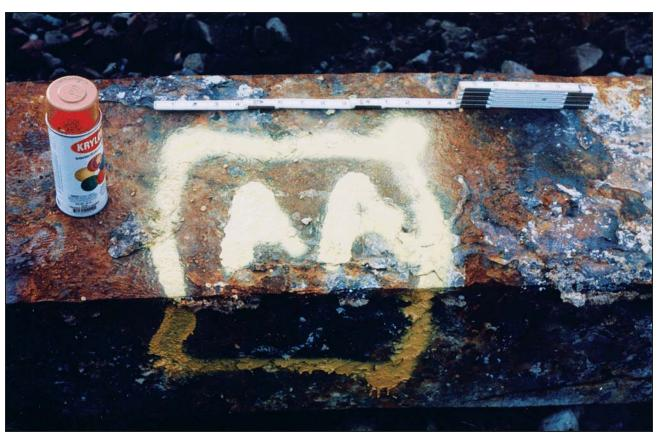
Figure D-11 Burnt steel piece marked for cutting of coupon.
