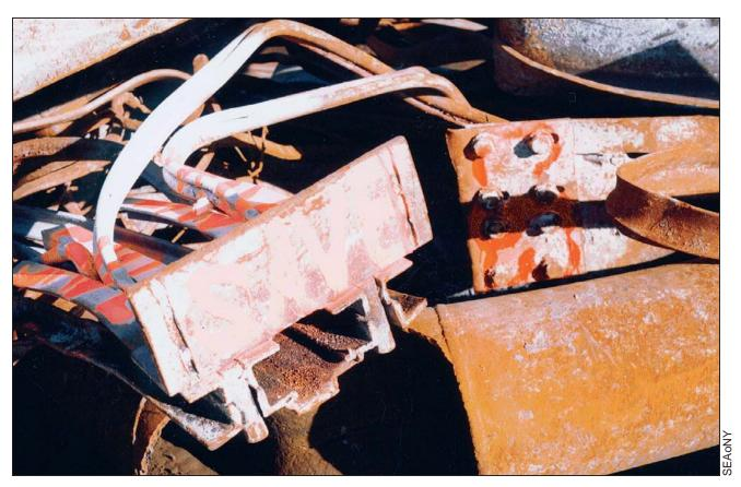
Figure D-18 WTC 1 or WTC 2 floor-truss section with seat connection fractured along welds.
