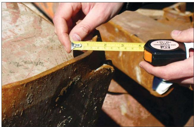
Figure D-9 Measurement of 1/4 inch for web thickness (t,,).
