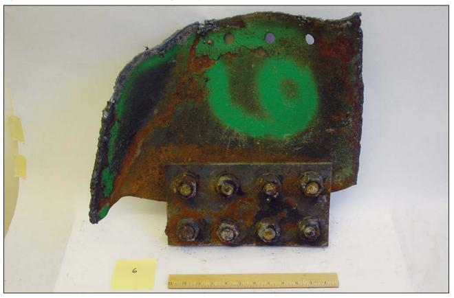
Figure D-12 Coupon cut from WTC 5 showing web tear-out at bolts.
