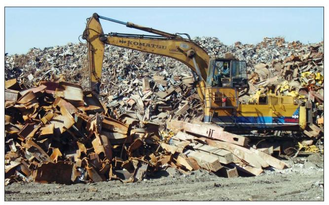
Figure D-3 Pile of unsorted, mixed steel (background) with sorted, large steel pieces (center) being lifted and cut into smaller pieces (left).
