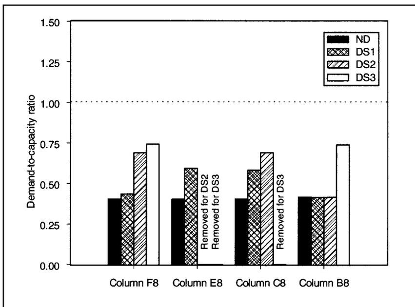
Figure 3.6. Demand-to-capacity ratios for three-dimensional linear elastic analysis
