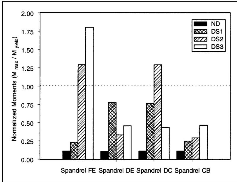
Figure 3.3. Demand-to-capacity ratios for two-dimensional linear elastic analysis
