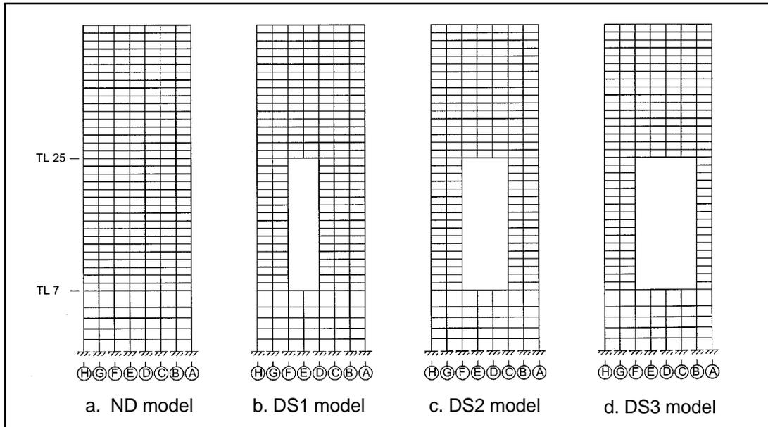
Figure 3.1. Two-dimensional mathematical models of framing on Line 8
