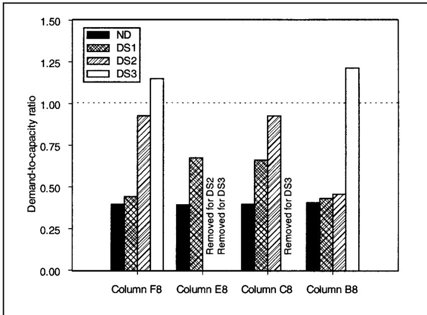
Figure 3.5. Demand-to-capacity ratios for two-dimensional linear elastic analysis
