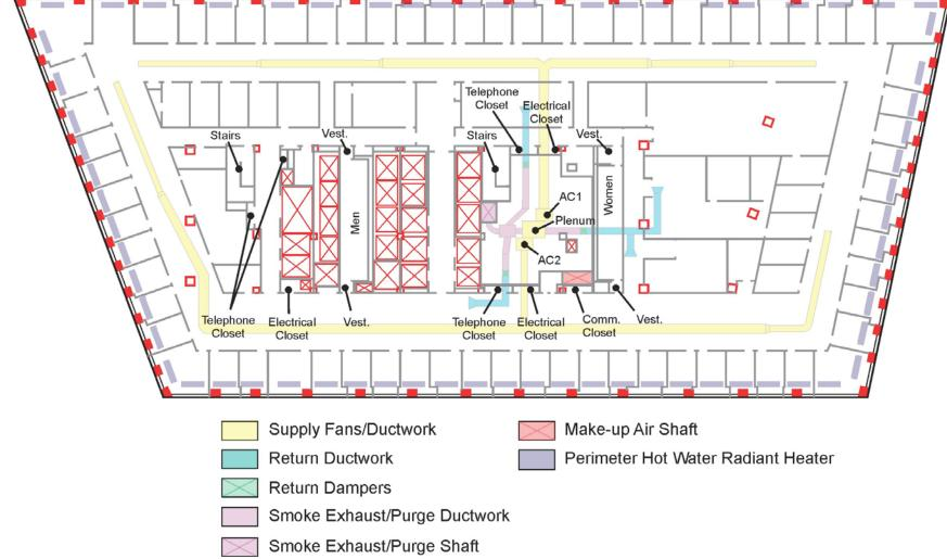
Figure 5–6. Air distribution system, 24th floor, WTC 7.
