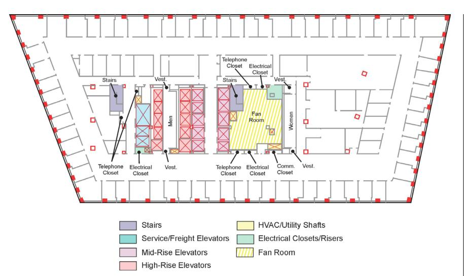
Figure 5–5. Floor layout, 24th floor, WTC 7.
