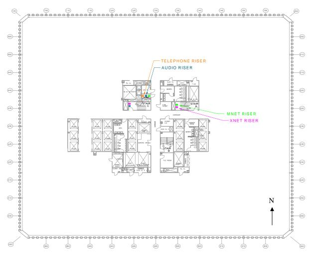
Figure 4–8. Typical WTC 1 riser locations on impact floors.
