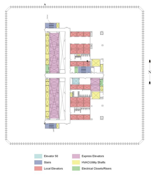
Figure 5–3. Floor layout, 80th Floor, WTC 2, South Tower.
