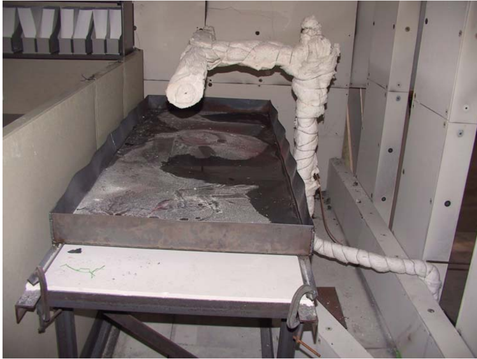
Figure 2–9. Spray burner and fire pan abutting Workstation 1 before Test 2 (location B1).
