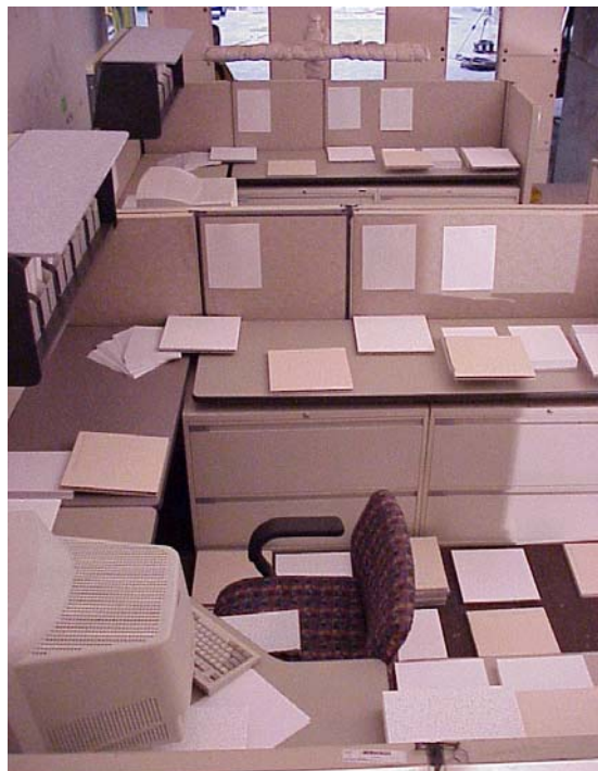
Figure 2–6. Image highlighting the arrangement of ceiling tiles used in Tests 3 and 4. The spray burner and compartment openings are visible towards the rear.
