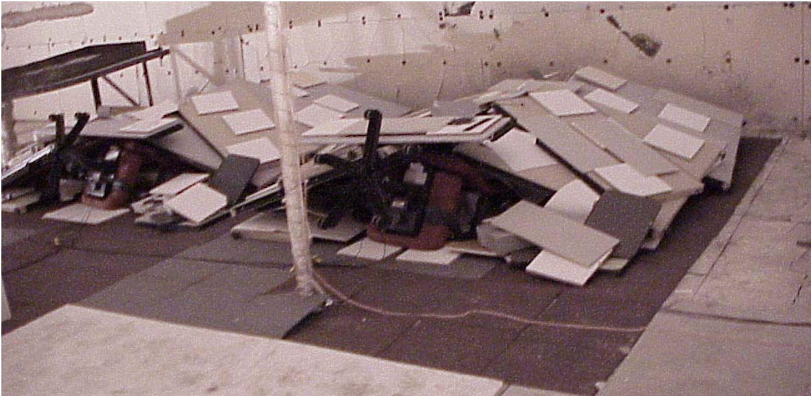
Figure 2-7. The arrangement of “rubblized” Workstations 1 (left) and 2 (right) with ceiling tiles before Test 5. Part of the spray burner is visible on the left.
