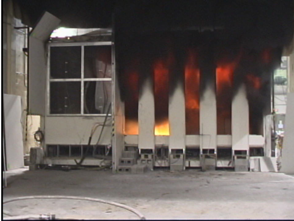
Figure 3–10. View external to the compartment 30 s after ignition of the spray burner in Test 6.
