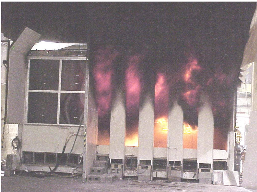
Figure 3–4. View of fire compartment 2 min after the start of Test 6.
