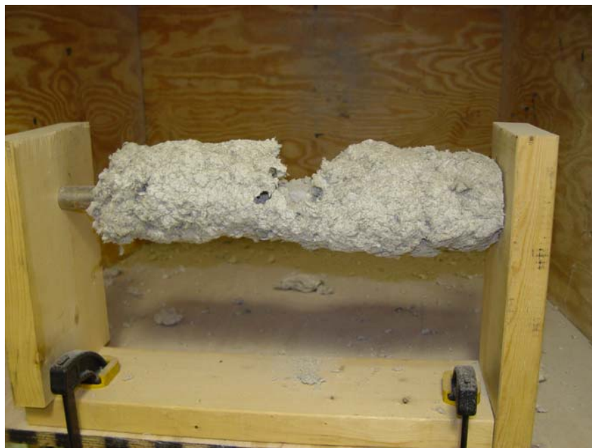
Figure C-9. Photograph showing damage to the SFRM on an unprimed steel bar (BAR01) after a ballistic impact at 0 degree using the small universal receiver.
