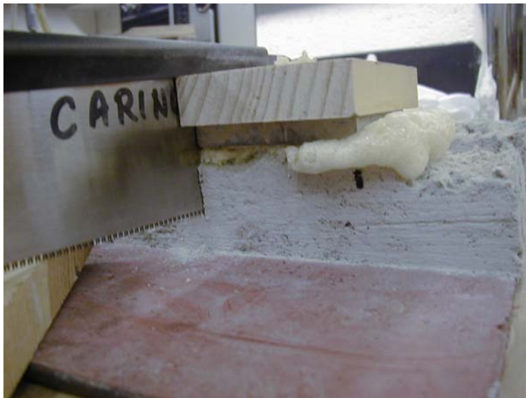
Figure 7–12. Preparing the SFRM specimen for adhesion/cohesion test.
