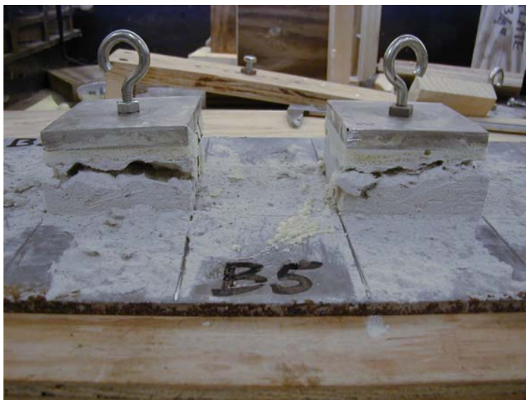
Figure 7–24. Examples of cohesive failure in 1½ in. SFRM specimens.
