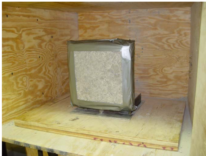
Figure C-7. Photograph showing damage to the SFRM after a ballistic impact at 60 degree. The SFRM layer did not separate from the steel plate.
