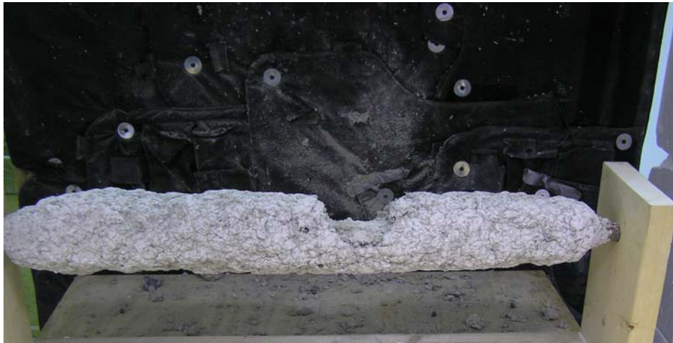
Figure C-12. Photograph showing damage to the SFRM on unprimed steel bar (BAR05) after a debris impact at 0 degree using the large universal receiver.
