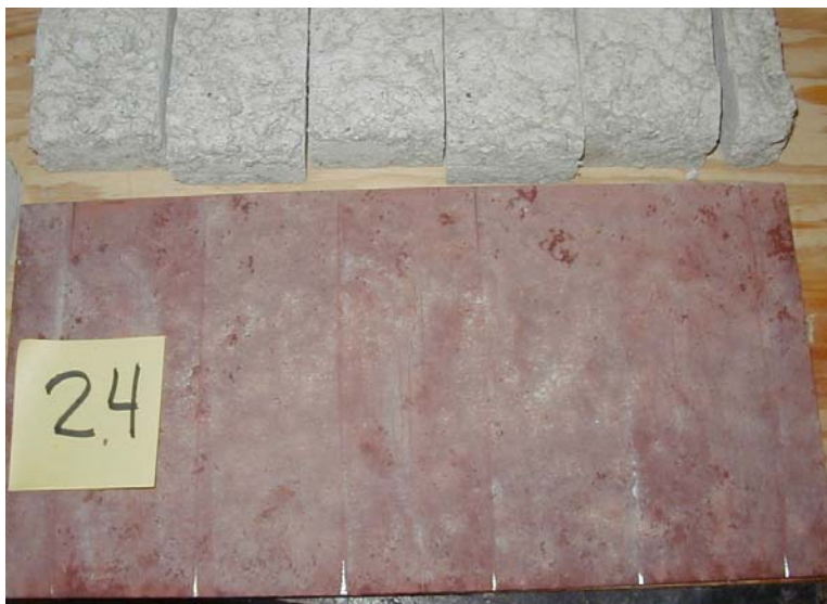
Figure 7–21. Example of lack of adhesion in 1½ in. SFRM on steel plate with primer.
