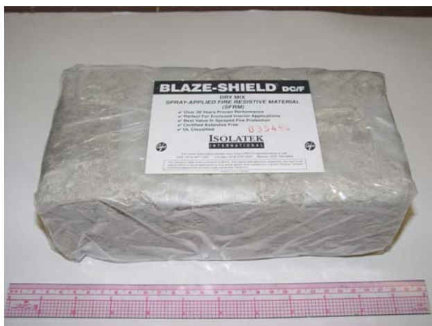
Figure 6–1. BLAZE-SHIELD DC/F sample used for thermophysical property measurements.
