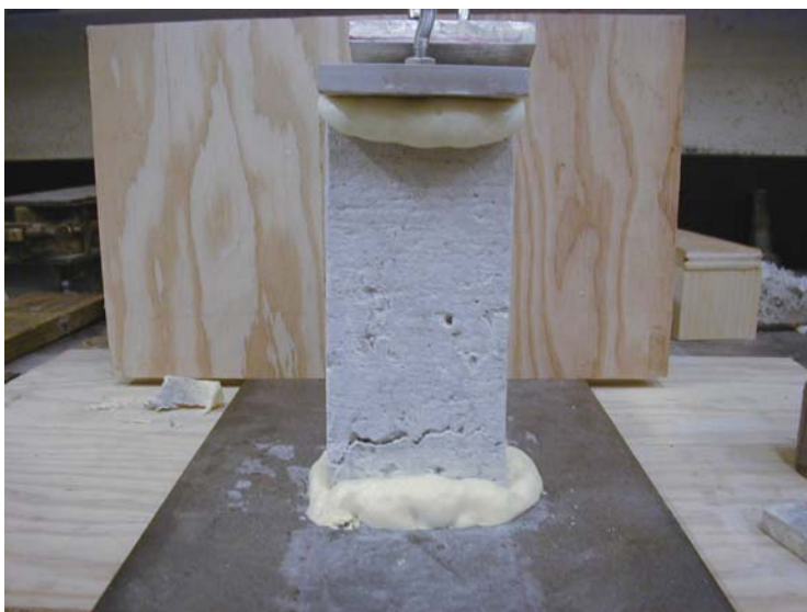
Figure 7–16. SFRM specimen after measuring in-plane cohesive strength.
