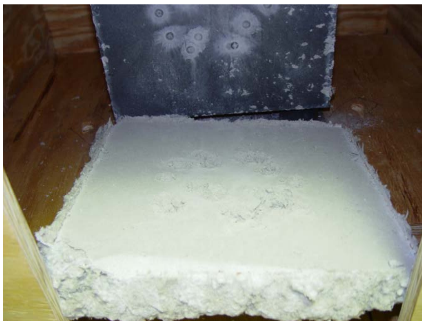
Figure C-4. Photograph showing damage to the SFRM after a ballistic impact at 0 degree. The SFRM layer completely separated from the steel plate.
