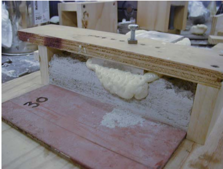
Figure 7–11. Aluminum plate being bonded to the top surface of SFRM specimen; the wooden fixture is used to maintain the correct alignment of the plate.
