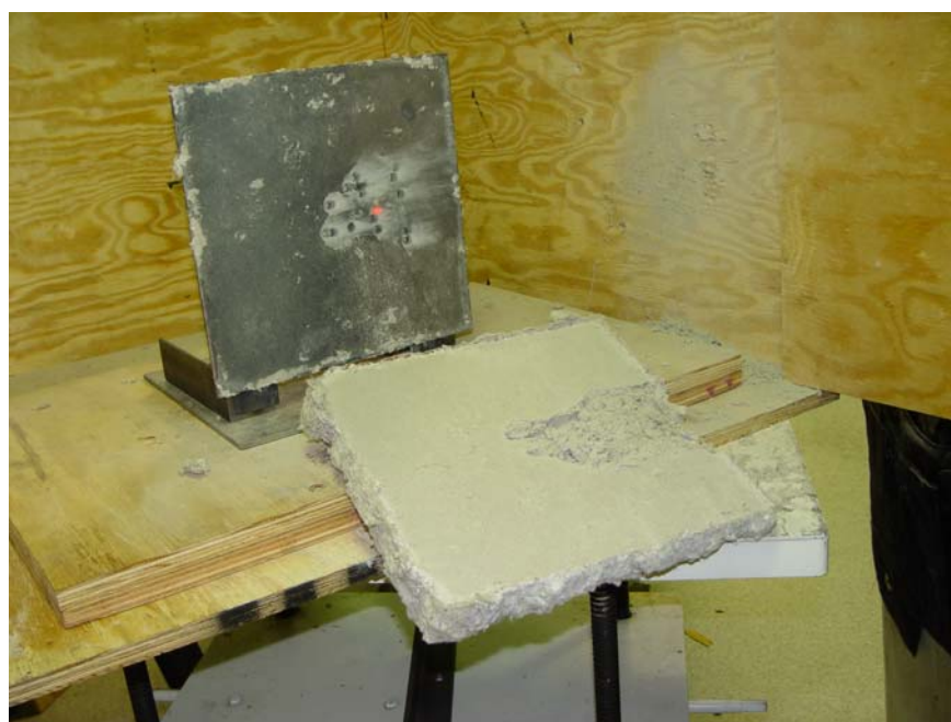
Figure C-5. Photograph showing damage to the SFRM after a ballistic impact at 20 degree. The SFRM layer completely separated from the steel plate and landed on the floor.
