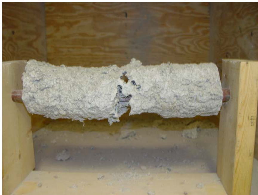
Figure C-10. Photograph showing damage to the SFRM on a primed steel bar (BAR02) after a ballistic impact at 0 degree using the small universal receiver.
