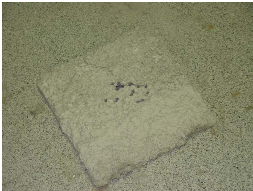
Figure C-5. Photograph showing damage to the SFRM after a ballistic impact at 20 degree. The SFRM layer completely separated from the steel plate and landed on the floor.
