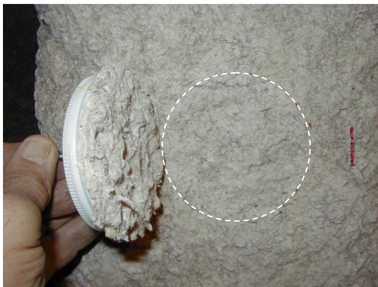
Figure 7–2. Cohesive failure of SFRM using ASTM E 736 test (dashed circle is approximate location of cap before being pulled off).
