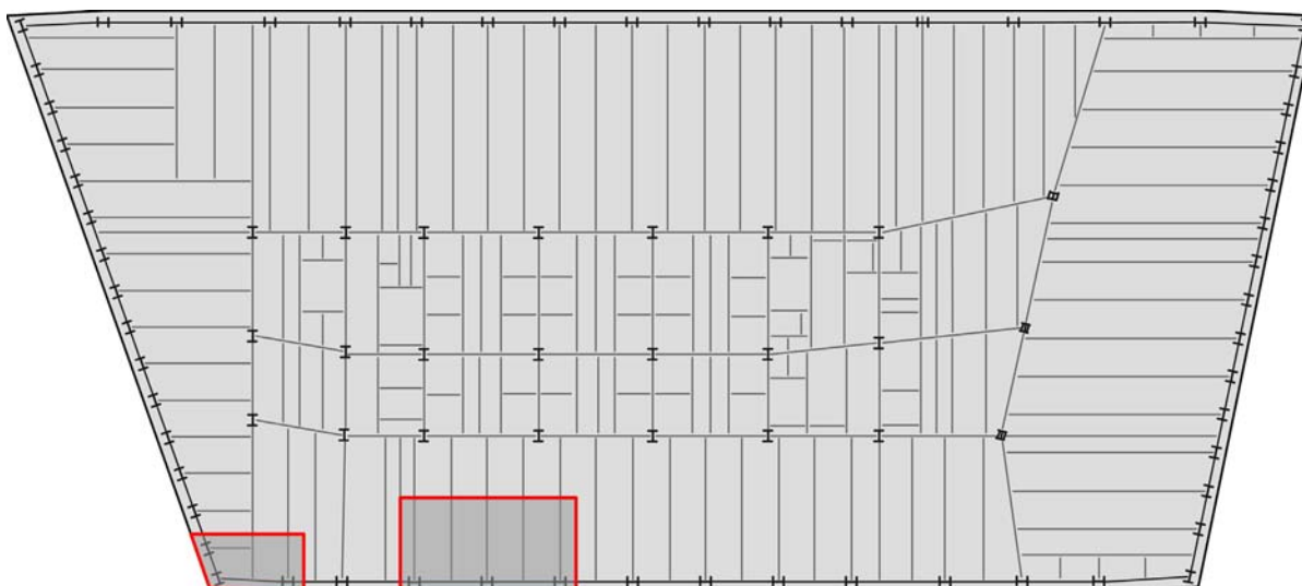
Figure 5–99 Estimated debris impact damage to Floors 12 to 14 of WTC 7.
