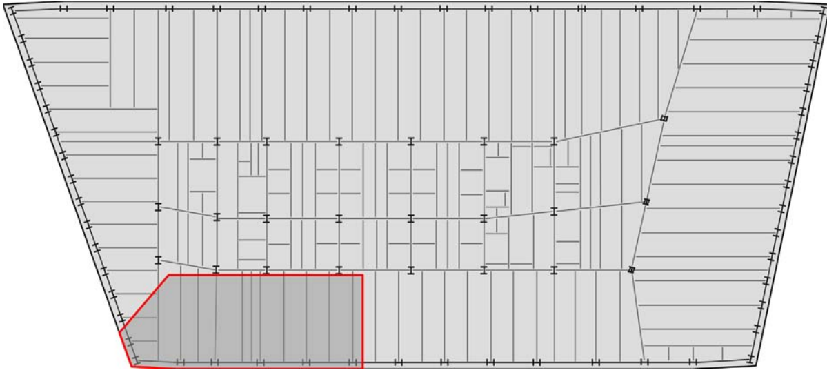
Figure 5–96 Estimated debris impact damage to Floor 8 of WTC 7.
