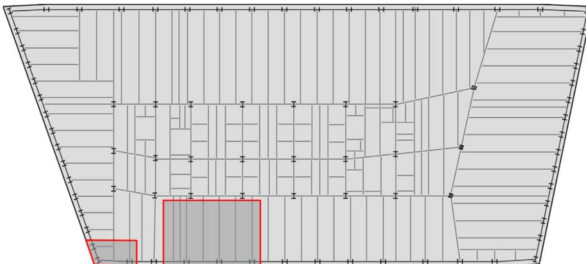
Figure 5–98 Estimated debris impact damage to Floors 10 and 11 of WTC 7.
