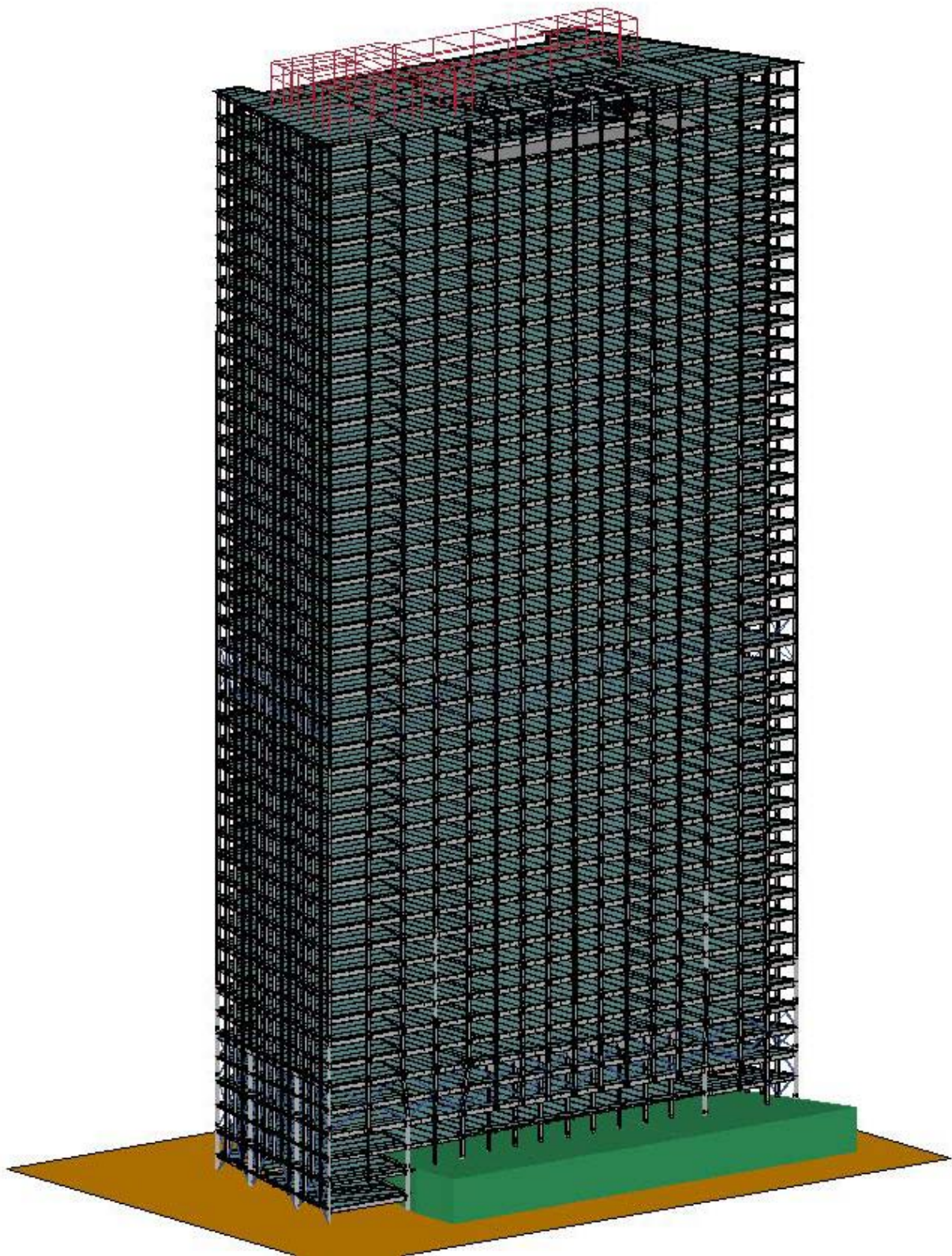
Figure 12–7. Global model of WTC 7, viewed from the northeast.
